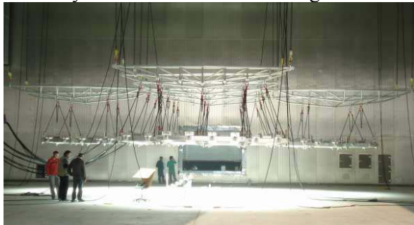
Fig. 3 Equipment support system with solar simulation system installed
