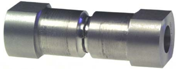
Fig. 7. Hollow test specimen with notch, which was subjected to tension. Fatigue tests were performed, hence the crack, these were however not the subject of this article.
