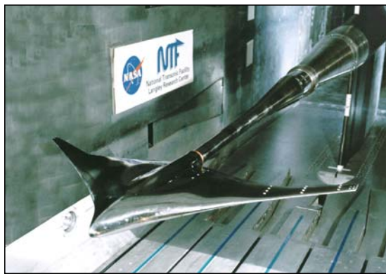
Figure 13 BWB in the NASA LaRC National Transonic Facility (NTF)
