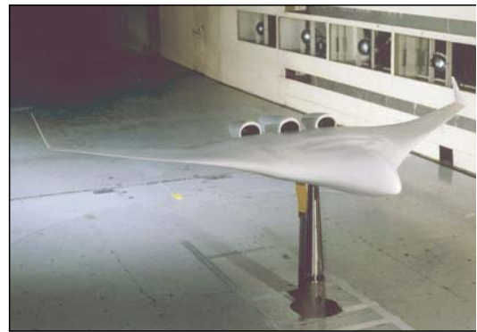
Figure 15 Powered BWB model in the NASA LaRC 14x22 foot tunnel for low-speed test.
