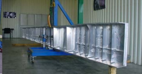
First Front Spars by Saab at Mecachrome
