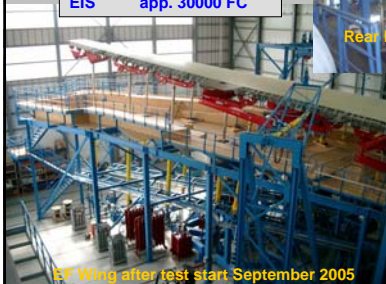
EF Wing after test start September 2005
