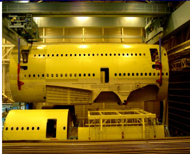
27/11/03 Centre section assembly from upper shells integration station to belly fairing installation station.
