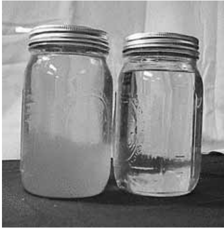
Figure 5. Biofuel (right) would need to be mixed at a maximum 20% ratio to avoid stability issues over time (left). [3]
