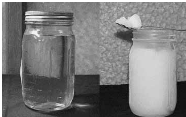
Figure 3. One issue to address is that regular bio-diesel fuel (left) freezes at the cold (i.e., -20\text{ }^\circ\text{C} ) operating conditions of aircraft (right). [3]
