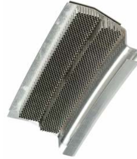
Figure 10. Outer Airseal With Low Cost Honeycombs
