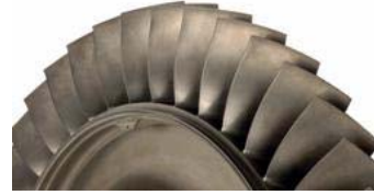
Figure 6: IBRs Replacing Bladed Rotors in JTDP02
