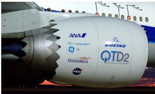
Fig 2. PAA T-fan chevrons and core chevrons
