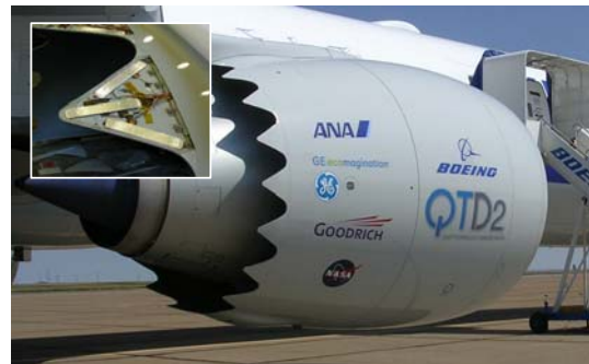
Fig 3. Variable geometry fan chevrons (inset shows individual chevron with cover removed)
