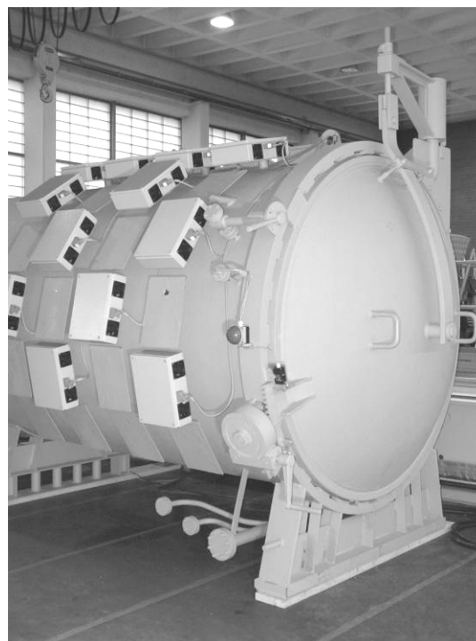
Fig. 17 Microwave autoclave at DLR/FA in the test phase
