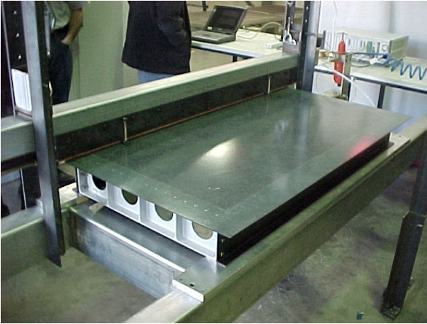
Fig. 9. Welding of Demonstrator Box
