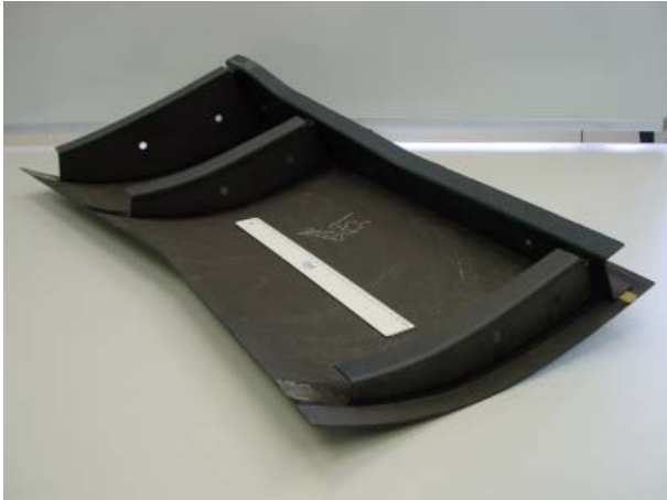
Fig. 12. Partially-Completed Flap Structure
