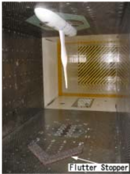
Fig. 8 Model installed in the wind tunnel test section
