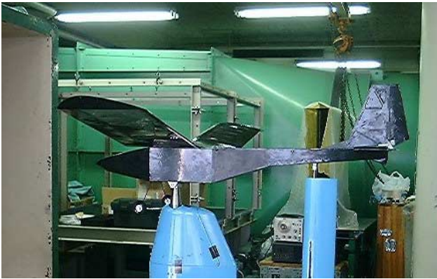
Fig. 5 70% Scale Model for Wind Tunnel Testing
