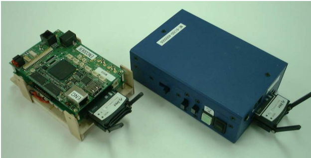
Fig. 9 Encoder and Decoder Equipped with Cellular Phone Cards
