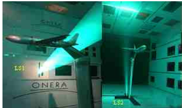
Fig. 19: Aircraft model to study wake survey in F1 wind tunnel by different techniques (5 holes probe, PIV, DGV)
