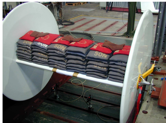
Fig. 3. Structural static test
