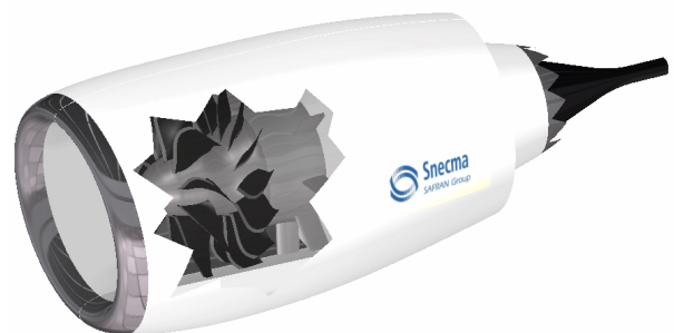
Fig. 4. CRTF engine ( Snecma Property )
