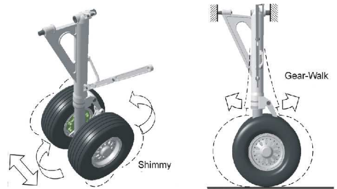
Fig. 1 Shimmy and Gear Walk [19]
