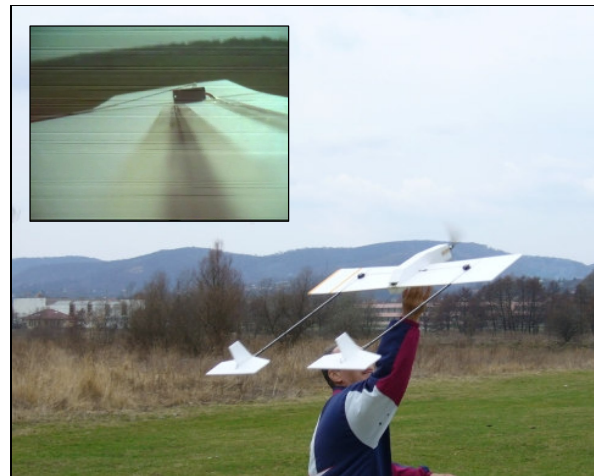
Fig. 9. RC model with active aeroelastic aileron control and onboard camera
