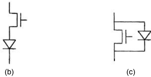
Fig. 6. (a) Schematic of RESEMI topology and switch definition for (b) source-side controller and (c) load-side controller.
