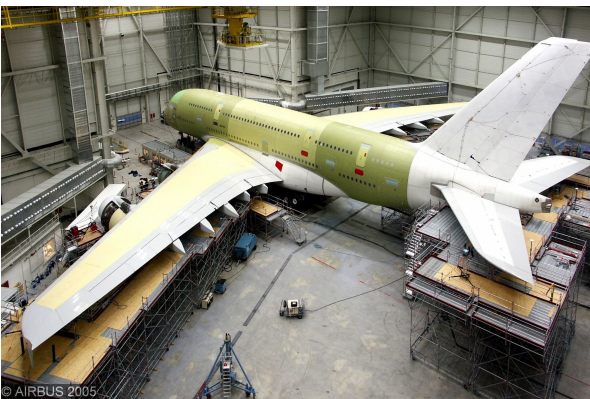
‘Fig. 9. A380 Ground Vibration Test’
