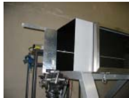
Fig. 8. Wind tunnel and position of wing model
