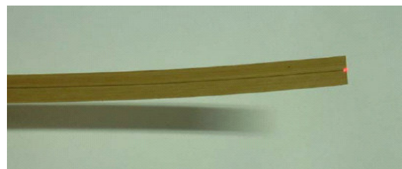
Fig. 4 Single mode optical fibre sensor (SMARTape) [11]
