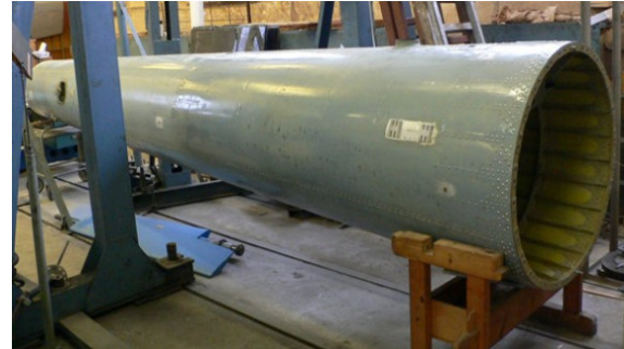
Fig. 2 Beam of a MI-8 helicopter selected for full-scale fatigue tests
