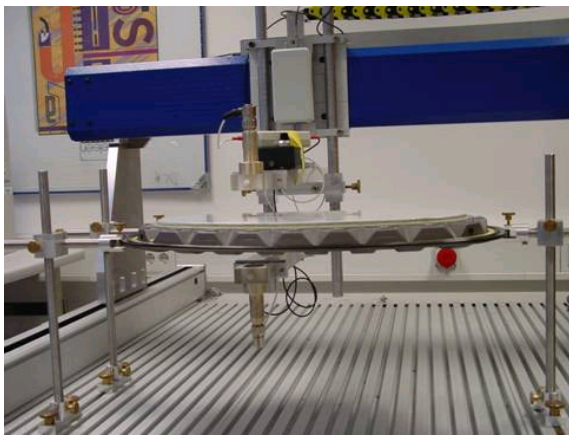
Fig. 3 Scanner system of the HFUS 2400 AirTech
