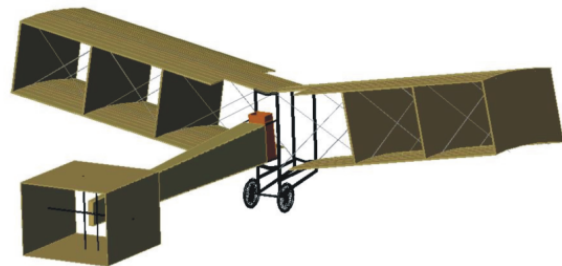
Fig. 2 Original CAD model (Source: EESC-USP).
