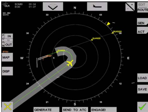
Fig. 7 Navigation Display as interface to the AFMS during a continuous descent approach
