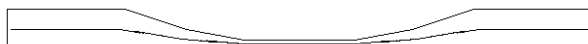
Cross section of 3D FE variable thickness shell model, showing how centerlines were offset, overlaid on drawing of solid cross section, for case 4.
