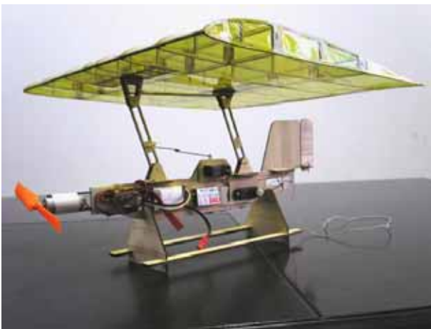
Fig.2. Layout of the MAV (with an underside bracket)
