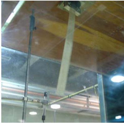
Fig. 7. Balsa wing static deflection
