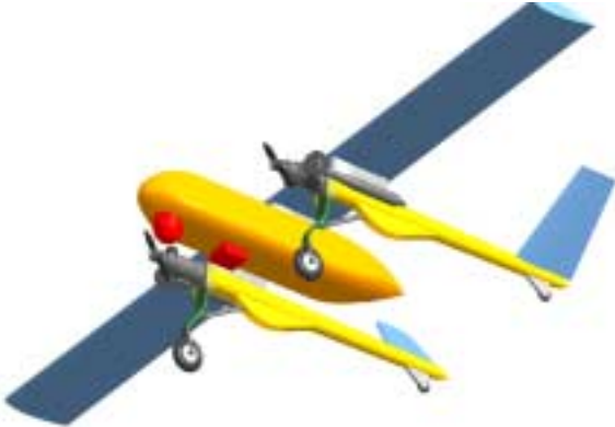
Fig.13. Front-bottom view of PW-141 – main landing gear and tail wheel is well shown
