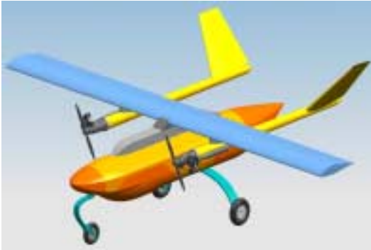
Fig.15. A modified version (PW-141B) with nose wheel and redesigned wing attachment
