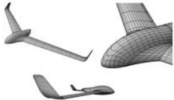
Fig.5. Meshes for panel methods calculation
