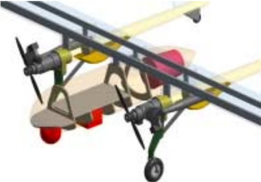
Fig.14. Frames of main container and wing spars
