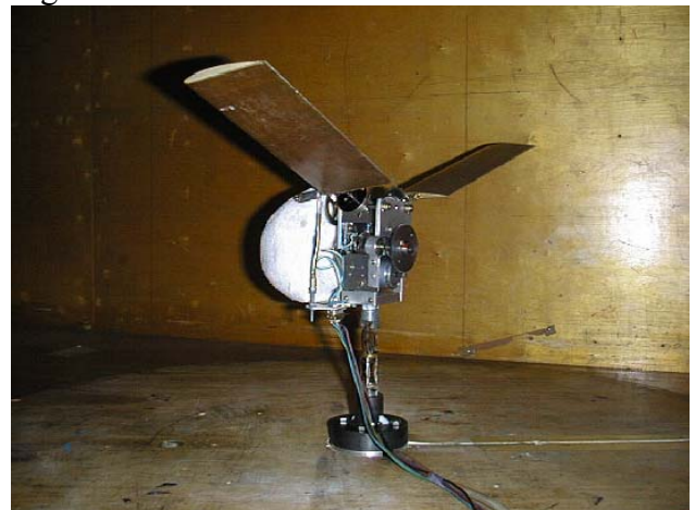
Fig. 5 Scheme of wind tunnel flapper [32].
