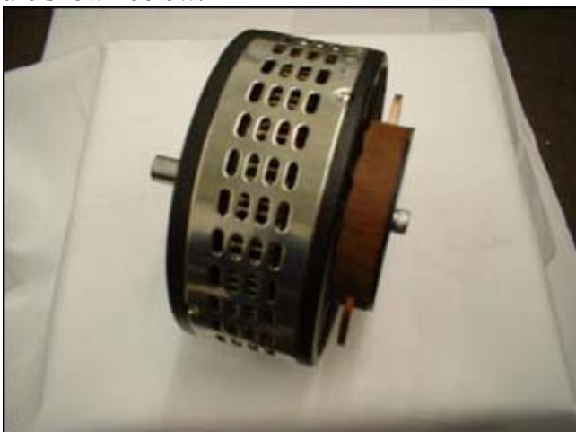
Fig 7a LMC brushed motor 3 kW, 3 kg, 6000 rpm
