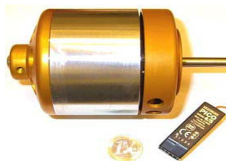
Fig 7c (Chosen) Torcman Monster 5.5 kW, 1.5 kg at 7000 rpm (www.torcman.de).
