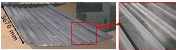
Fig. 31: Ageformed real size fuselage panel including pocketing, FSW and LBW stringers.
