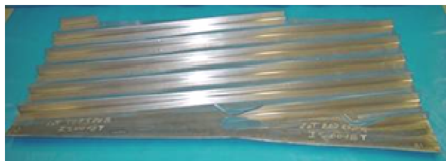
Fig. 39: Dassault break panel after ageforming.
