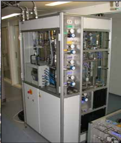
Test Rig with Reformer for SOFC Application
