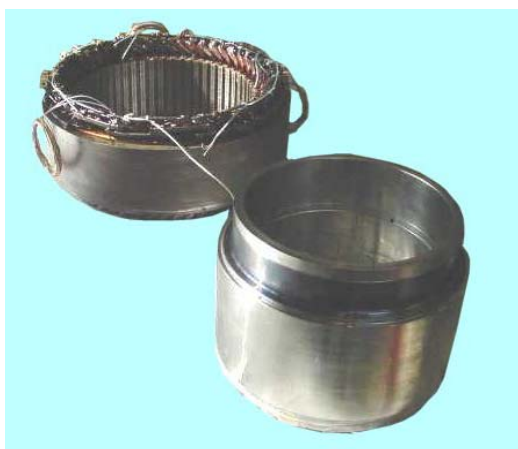
Fig. 2 - HPSG rotor (weight: 16 kg)
