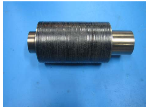
Fig. 17 – high speed permanent magnet rotor
