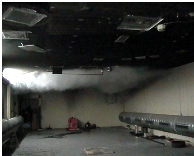
Fig. 6: Snapshot taken 30s after smoke emission by paraffin oil smoke generator (orange-coloured, center/bottom), the optical density meter can be seen in the center
