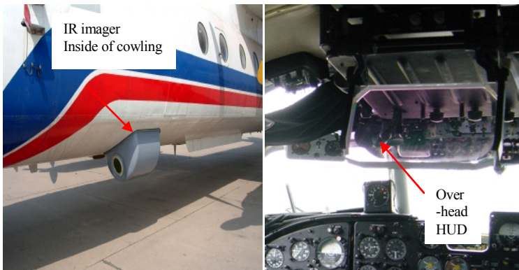
Fig.3 EVS Installed on Aircraft
