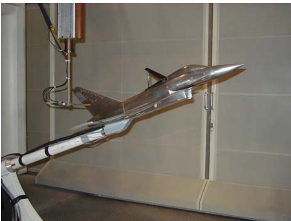
c) Model mounted in the test section
