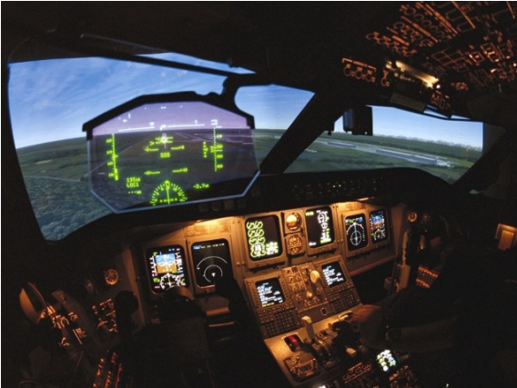
Fig. 2: View of the Canadair Jet-Flightdeck incl. HGS 2100 (Source: CST)
