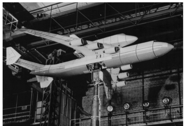
Fig. 9. Dynamically scaled model in WT T-104 TsAGI
