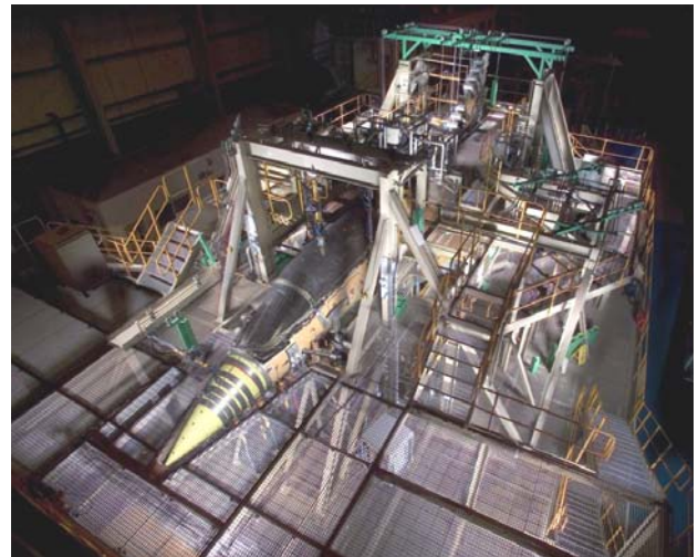
Fig. 16. Airframe structural tests
