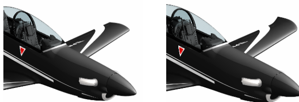
Figure 12: Original and up-swept wingtips
