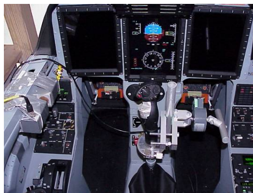
Figure 7: calibration of the control forces
