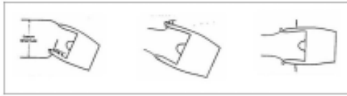
Low-speed windmilling high-speed cruising Fig.21. The key status of the nacelle in the integration of the wing and nacelle
