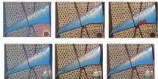
Fig.15. Test in T106 TsAGI wind tunnel, comparison oil flow visualization
