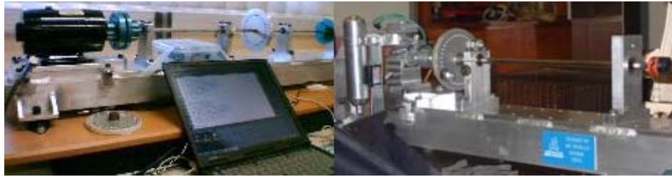
Fig. 7 Electric motor (left) and two-stroke motor (right) test setup
