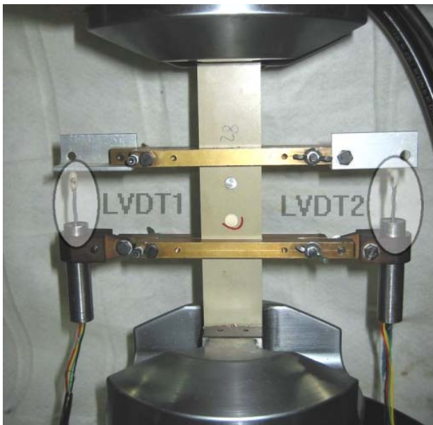
Figure 7. Test setup of two rivet row lap joint
