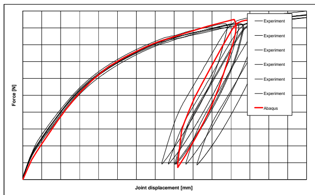
Figure 11. Load-displacement diagram of lock bolt lap joint test simulation
