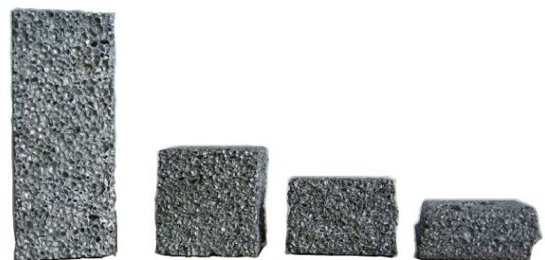
Fig. 3. Aluminium-Foam in different compression states
