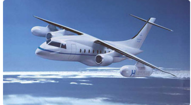
Fig.4 Conversion of a 328Jet [8]
