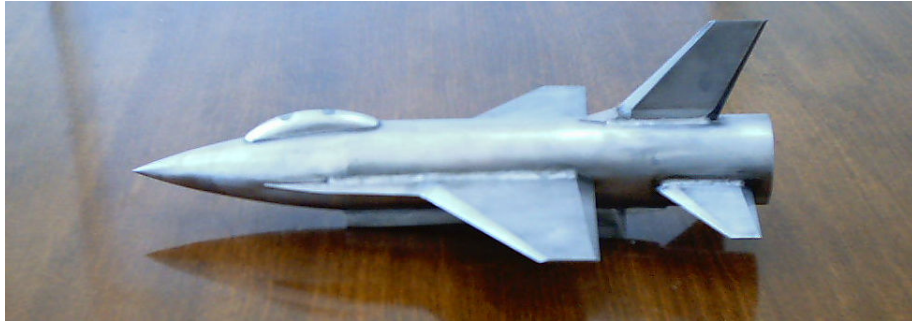
Figure 1- The Standard Dynamics Model (SDM) used in the present experiments
