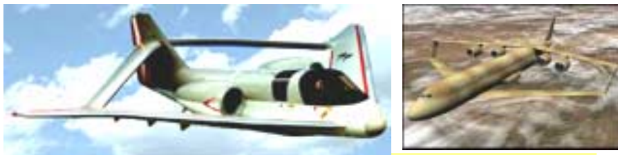
FIG. 2 SEVERAL RECENT JOINED-WING APPLICATIONS
