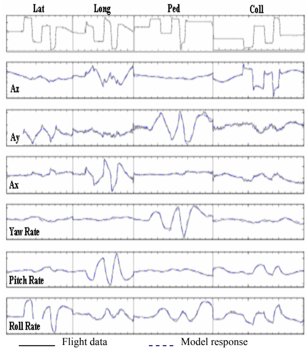
Fig. 3. Autorotation point model response at 60 kts for heavy/aft configuration
