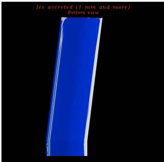
Figure 7 Ice accretion on 3-D wing in freestream – bottom view
