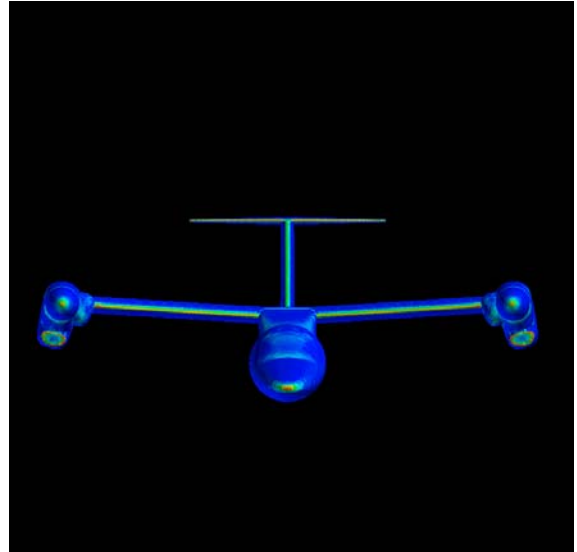
Figure 16 Collection efficiency on complete tiltrotor aircraft without rotors
