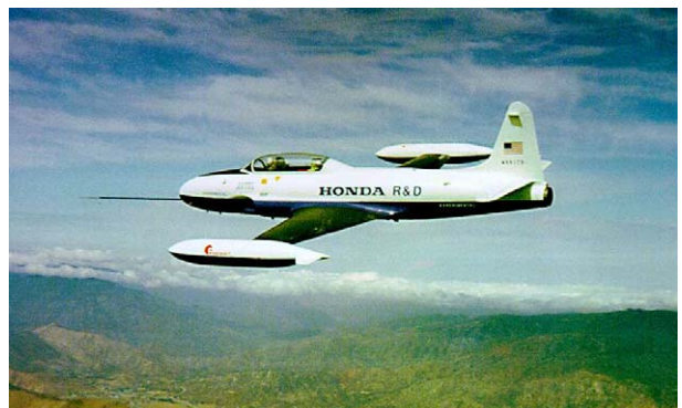
Fig. 9. T-33 aircraft modified for NLF flight test.
