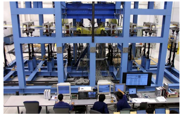
Fig. 32. Wing proof test.
