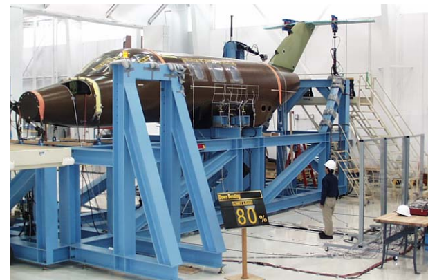
Fig. 33. Fuselage proof test.
