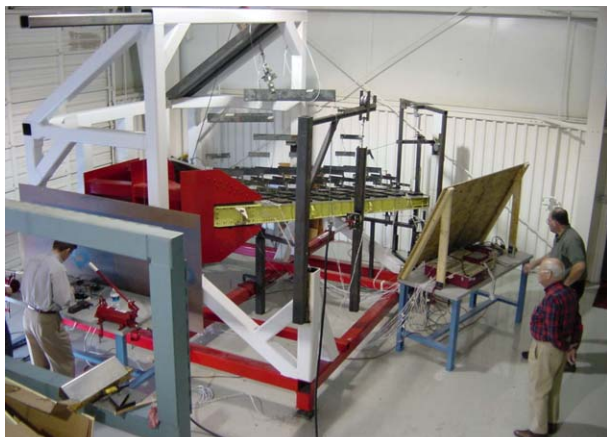
Fig. 35. Empennage proof test.
