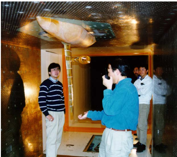
Fig. 21. Transonic wind tunnel flutter test at NAL transonic wind tunnel.
