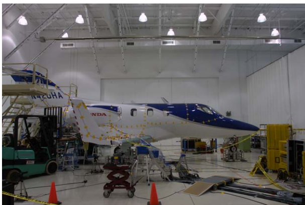
Fig. 37. Ground Vibration Test.
