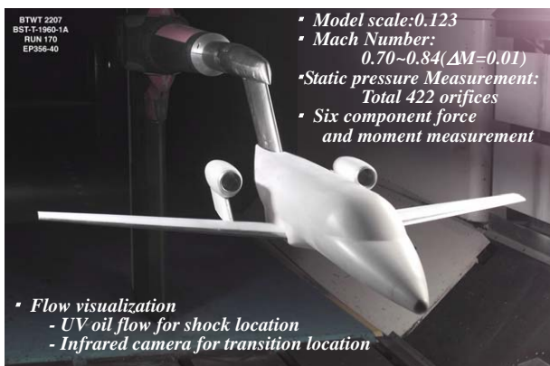
Fig. 5. Transonic wind tunnel test model (BTWT).
