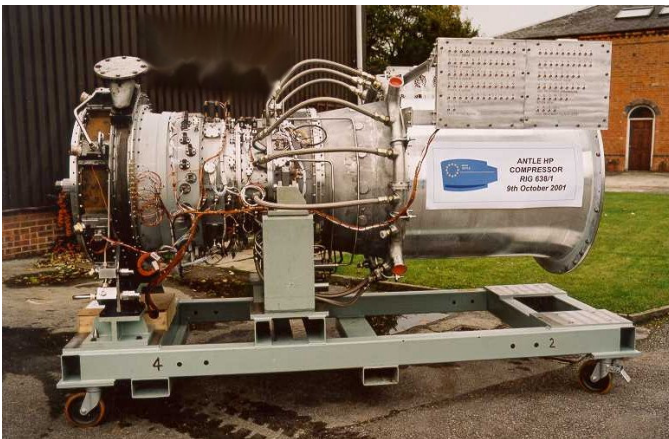
Fig. 3. ANTLE HP compressor rig
