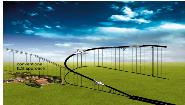
Fig. 5: Continuous Descent Approach (avoiding community) compared with conventional approach
